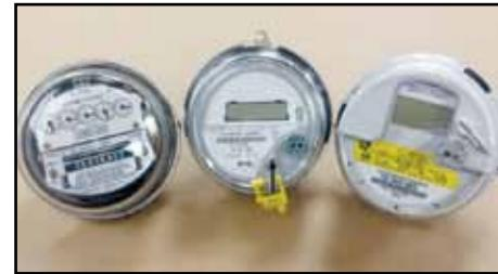
Consumers Energy has upgraded meter technology for residential customers and small businesses from electromechanical meters (left) to digital meters (middle) over the past 10 years, as the older meters have required replacement. Smart meters (right) have upgraded functions and will be installed across the state through 2017.
